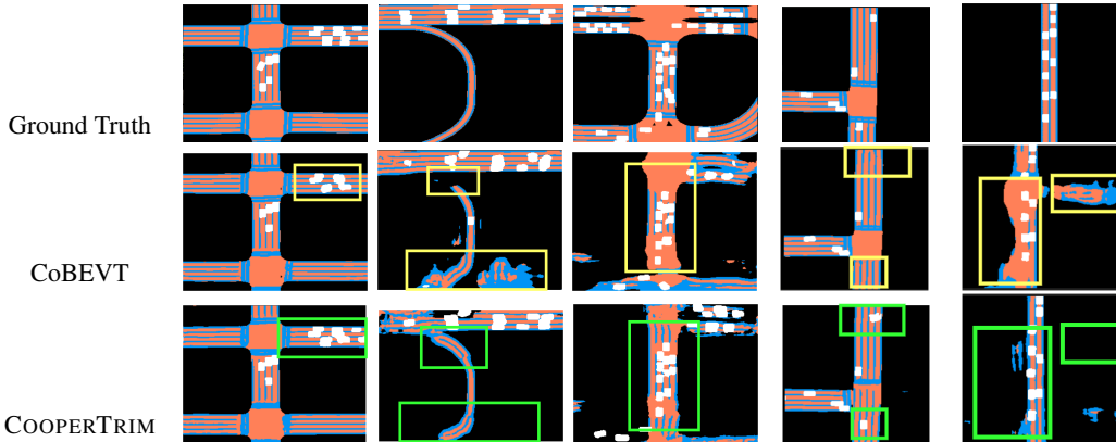
Figure 5: Qualitative Comparison of Ground Truth, CoBEVT, and COOPERTRIM. COOPERTRIM performs better than CoBEVT in estimating dynamic object segments (Column 1 and 4), road segments (Column 2 and 5), and lane segments (Column 3 and 5).
